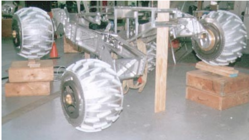
FIGURE 4-8: Nomad's Pitch Articulated Chassis
